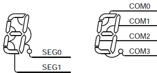
Figure11.5 The example of 1/4 duty (1/3 bias) LCD
